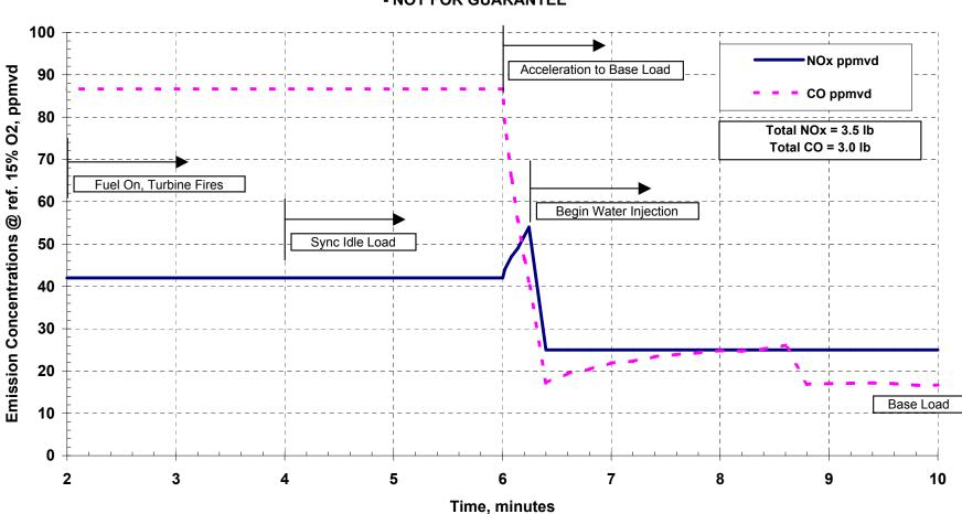
Estimated NOx and CO Concentrations during 10-Minute Startup at ISO Conditions - LM6000PC SPRINT - NOT FOR GUARANTEE
