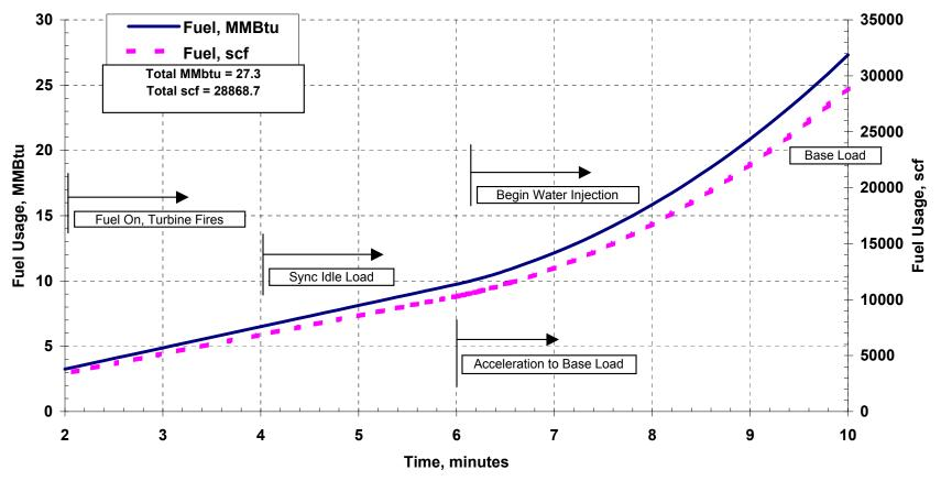
Acceleration to base load is based on 10 minute startup, Simple Cycle Operation, 59.0°F, RH of 60.0% with 5.0 inH2O, 10.0 inH2O at 0.0ft. MSL, Fuel: Gas Fuel #10-1, 19000 Btu/lb,LHV, Water NOx control to 25ppmvd. Water Injection starts at ~3000kW. BDAX 290ERT 60Hz, 13.8kV, 0.9PF (14839). NOT FOR GUARANTEE
