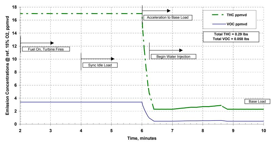
Estimated THC and VOC Concentrations during 10-Minute Startup at ISO Conditions - LM6000PC SPRINT - NOT FOR GUARANTEE
