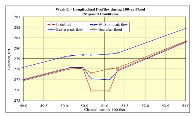
Fig. 18. Water-surface and channel bed profile changes during 100-yr flood for Wash C – proposed conditions with road crossings and sediment basins
