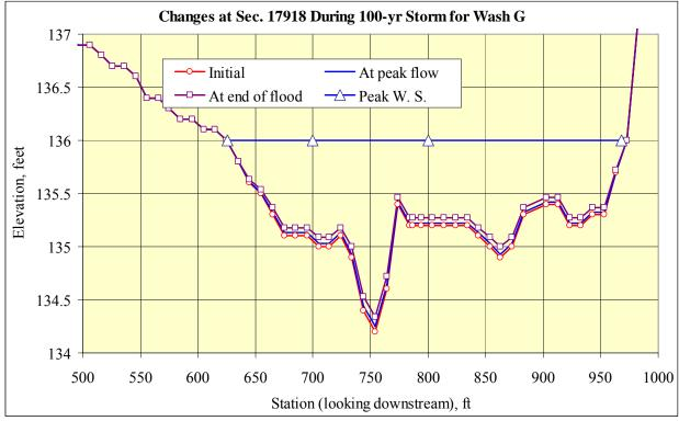
Fig. 30. Sample cross-sectional changes – proposed conditions with road crossings and sediment basins
