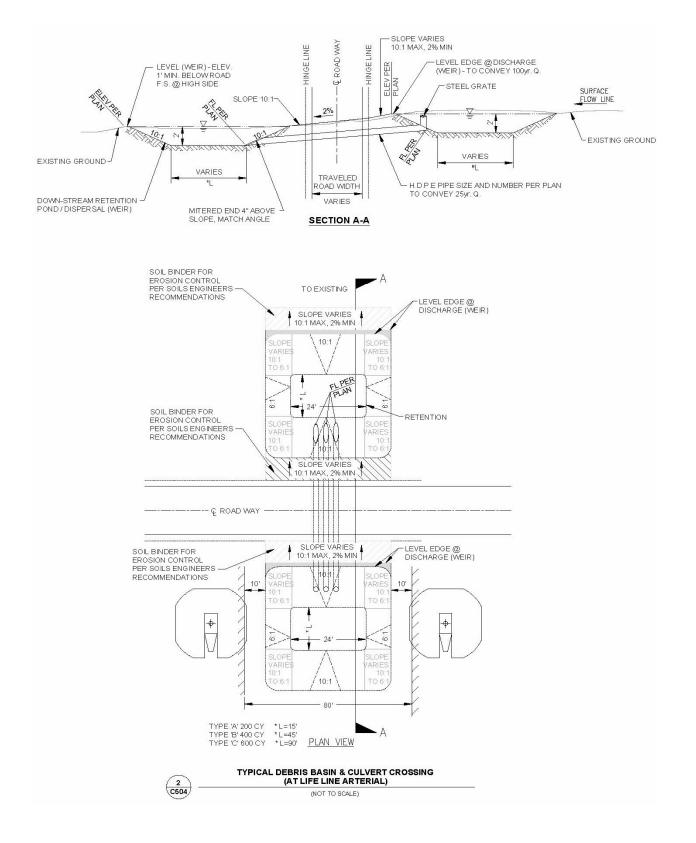
Fig. 4. Engineering plans for sediment basins
