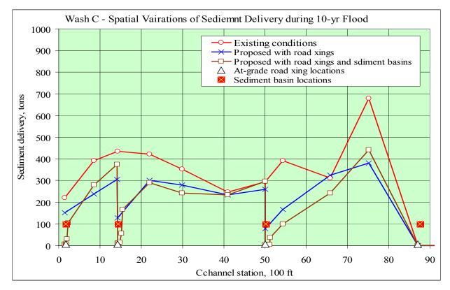
Fig. 22. Spatial variations of sediment deliveries during 10-yr flood for Wash C
