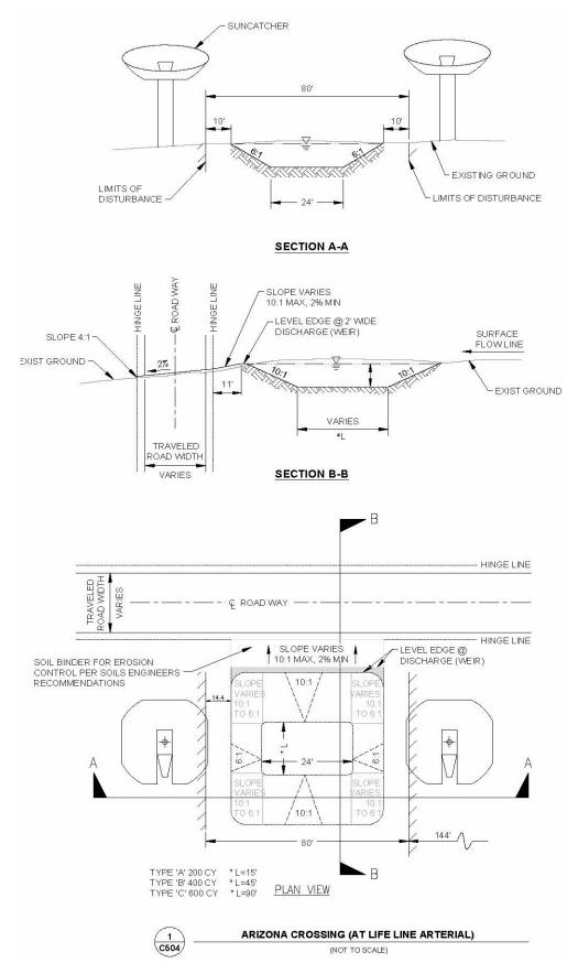
Fig. 5. Engineering plans for sediment basins
