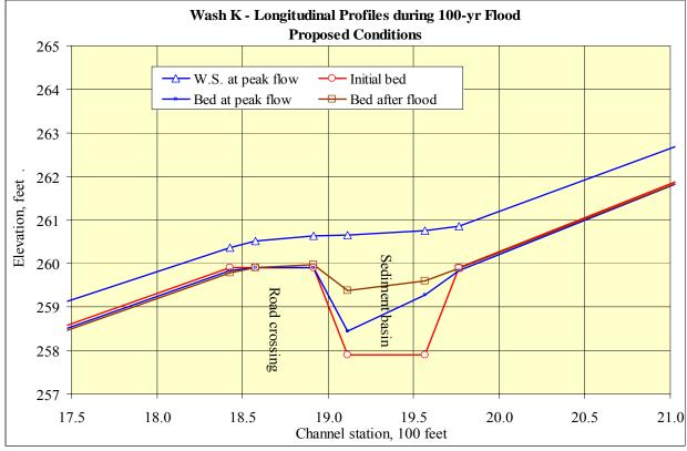
Fig. 11. Water-surface and channel bed profile changes during 100-yr flood for Wash K – proposed conditions with road crossings and sediment basins
