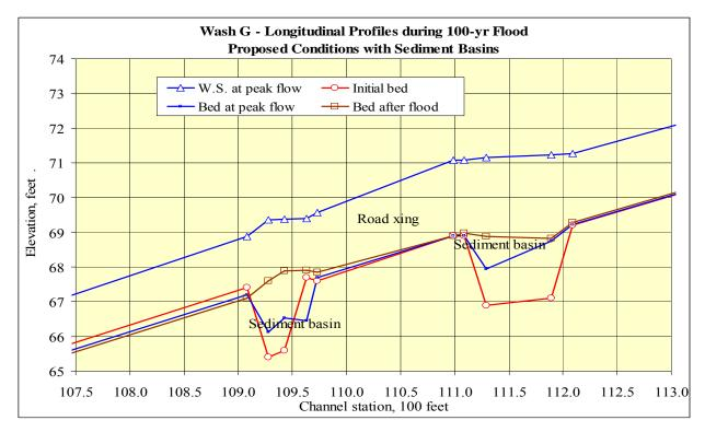
Fig. 29. Water-surface and channel bed profile changes during 100-yr flood for Wash C – proposed conditions with road crossings and sediment basins
