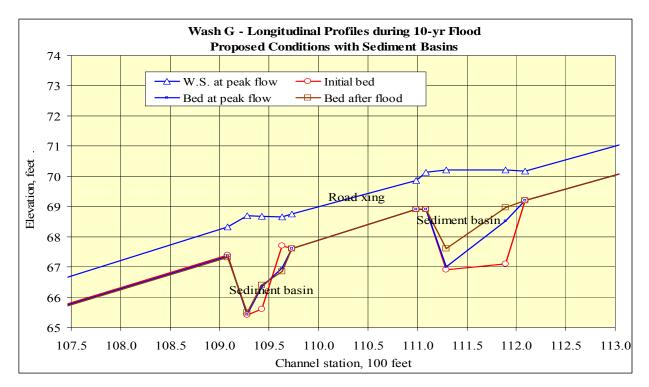
Fig. 28. Water-surface and channel bed profile changes during 10-yr flood for Wash G – proposed conditions with road crossings and sediment basins
