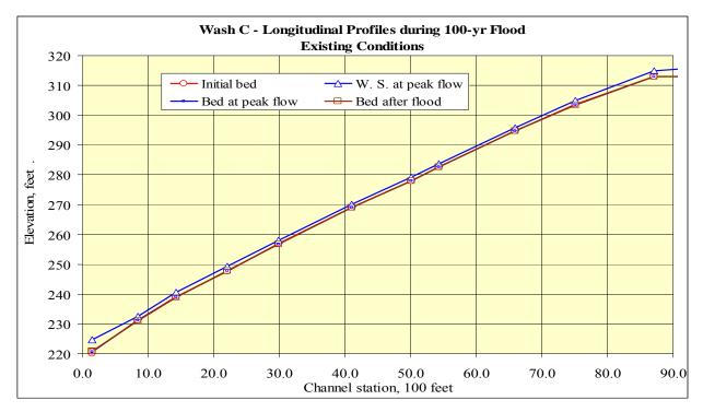
Fig. 16. Water-surface and channel bed profile changes during 100-yr flood for Wash C – existing conditions
