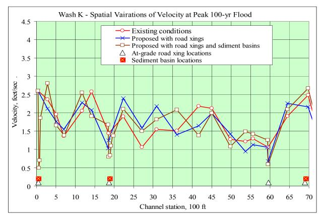
Fig. 13. Spatial variations of flow velocity at peak 100-yr flood for existing and proposed conditions
