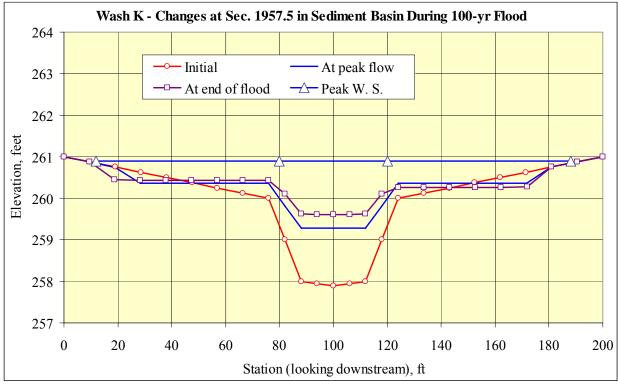
Fig. 12. Sample cross-sectional changes near sediment basin
