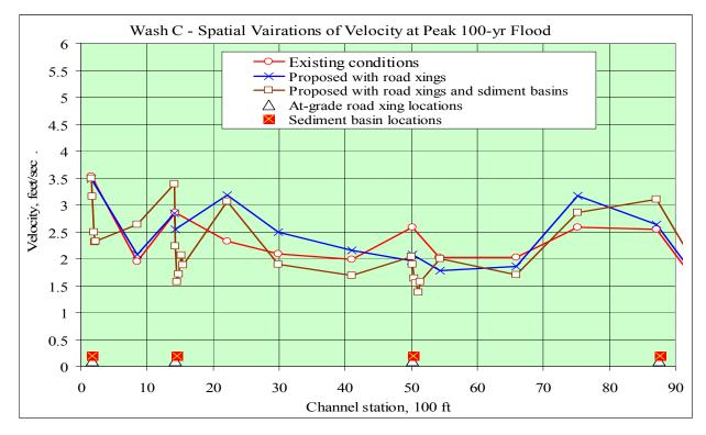
Fig. 21. Spatial variations of flow velocity at peak 100-yr flood for existing and proposed conditions
