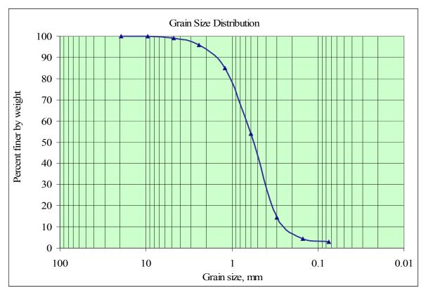
Fig. 3. Grain size distribution of sediment sample
