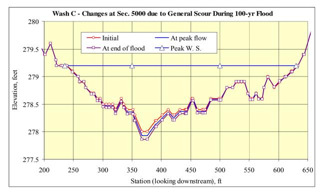
Fig. 19. Sample cross-sectional changes – proposed conditions with road crossings and sediment basins
