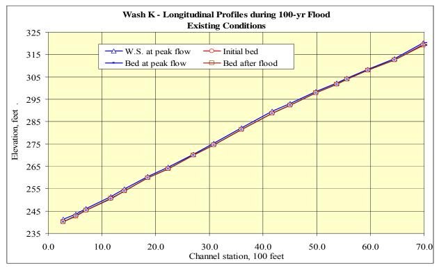
Fig. 9. Water-surface and channel bed profile changes during 100-yr flood for Wash K – existing conditions
