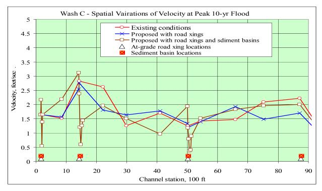
Fig. 20. Spatial variations of flow velocity at peak 10-yr flood for existing and proposed conditions
