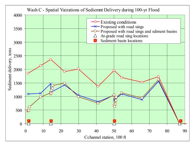
Fig. 23. Spatial variations of sediment deliveries during 100-yr flood for Wash C
