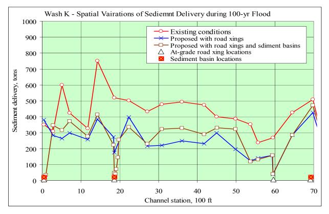
Fig. 14. Spatial variations of sediment deliveries during 100-yr flood for Wash K
