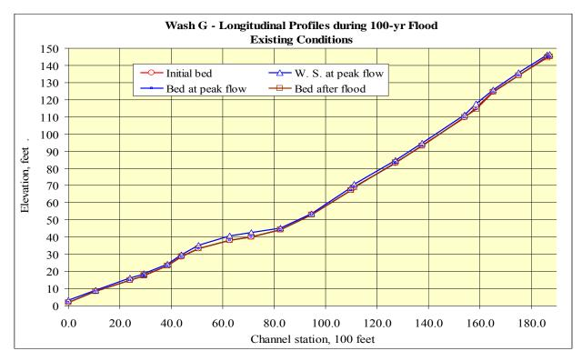
Fig. 26. Water-surface and channel bed profile changes during 100-yr flood for Wash C – existing conditions
