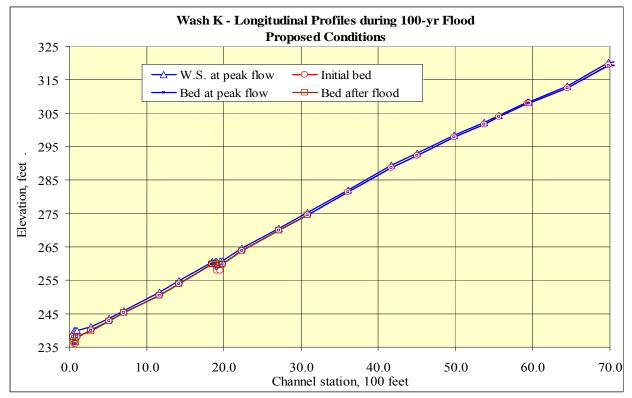
Fig. 10. Water-surface and channel bed profile changes during 100-yr flood for Wash K – proposed conditions with road crossings and sediment basins
