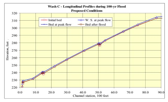
Fig. 17. Water-surface and channel bed profile changes during 100-yr flood for Wash C – proposed conditions with road crossings and sediment basins
