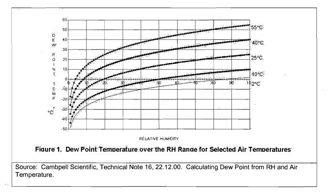
For projects in the desert such as the PHPP, ambient relative humidity can drop below 25% and so there will be a bias in CSVP due to the linearity assumption for these hours with low humidity. However, for many cases, this is not significant since under low humidity conditions, visible plumes are of lesser concern.
