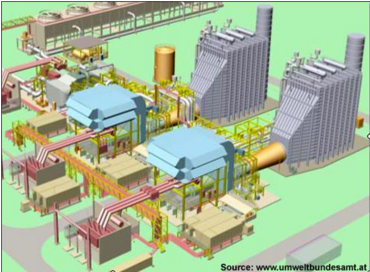
Figure C-4: Combined Cycle Power Plant General Arrangement
