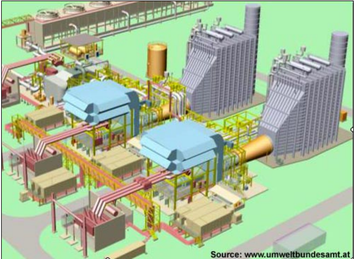
Figure C-4: Combined Cycle Power Plant General Arrangement
