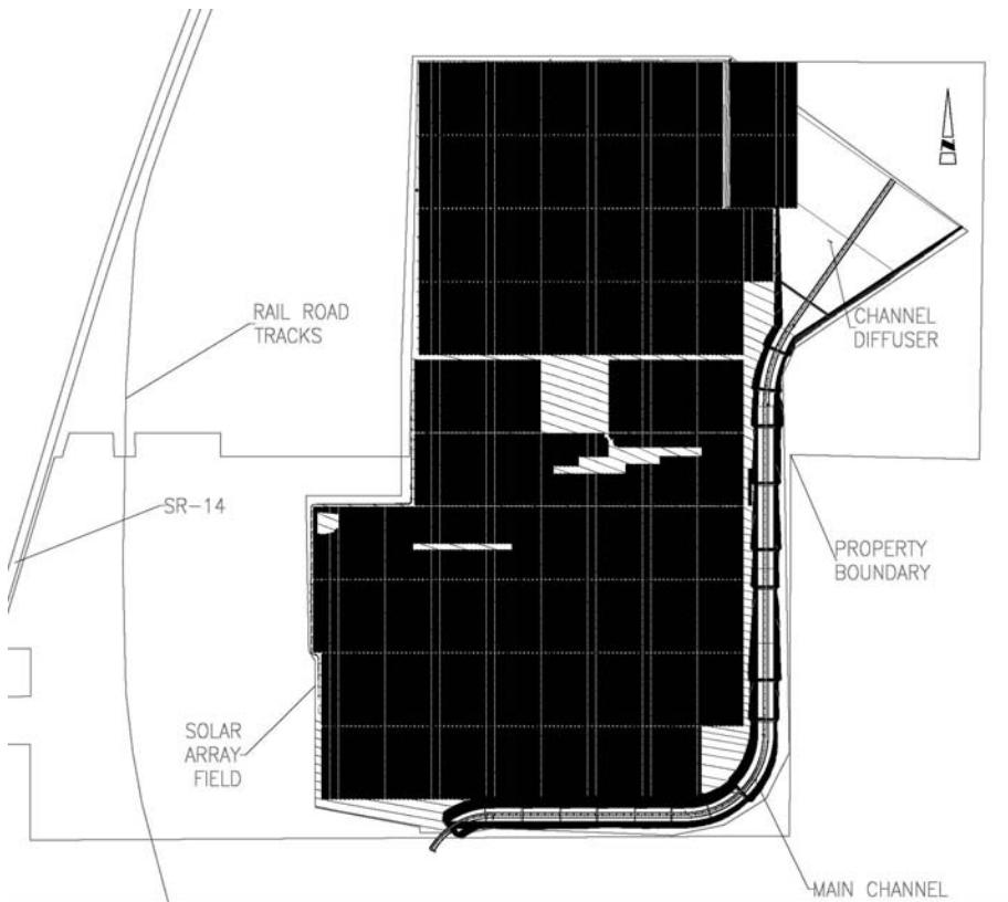
Fig. 1 Site Layout and Channel Concept
