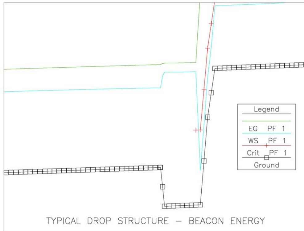
Fig. 2 HEC-RAS Drop Structure Water Surface Profile
