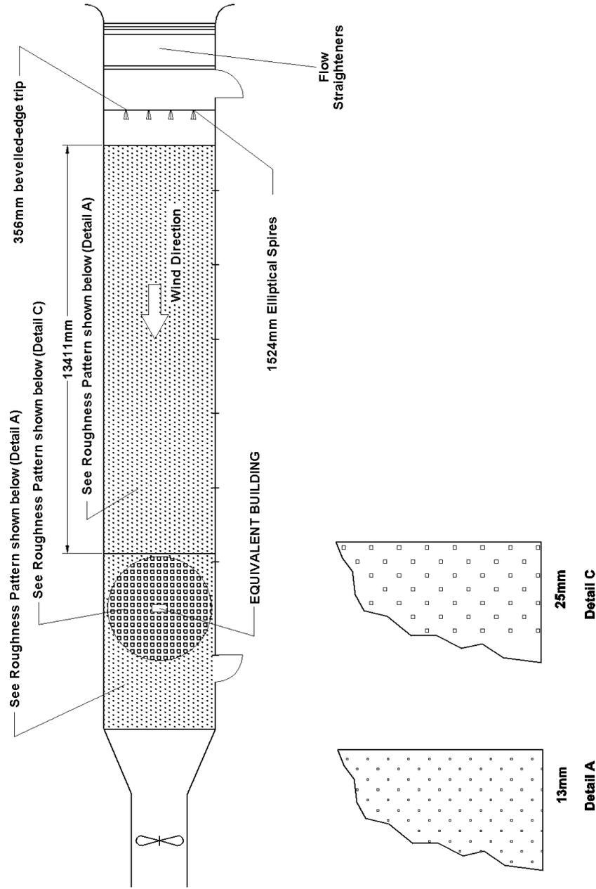
Figure 6. Wind tunnel setup for: c) tests with equivalent buildings - low roughness approach.
