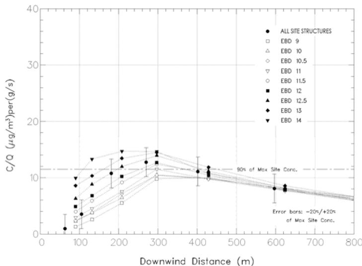
**Figure 3. Typical Ground Level EBD Results for BS4**
