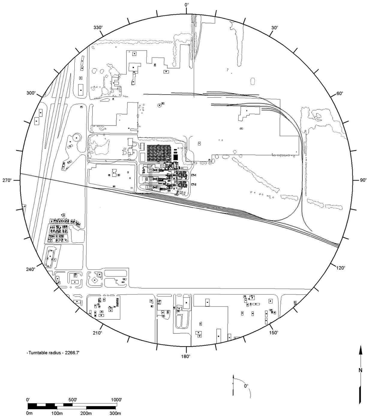
Figure 5. a) Site Plan of the area modeled in the wind tunnel.
