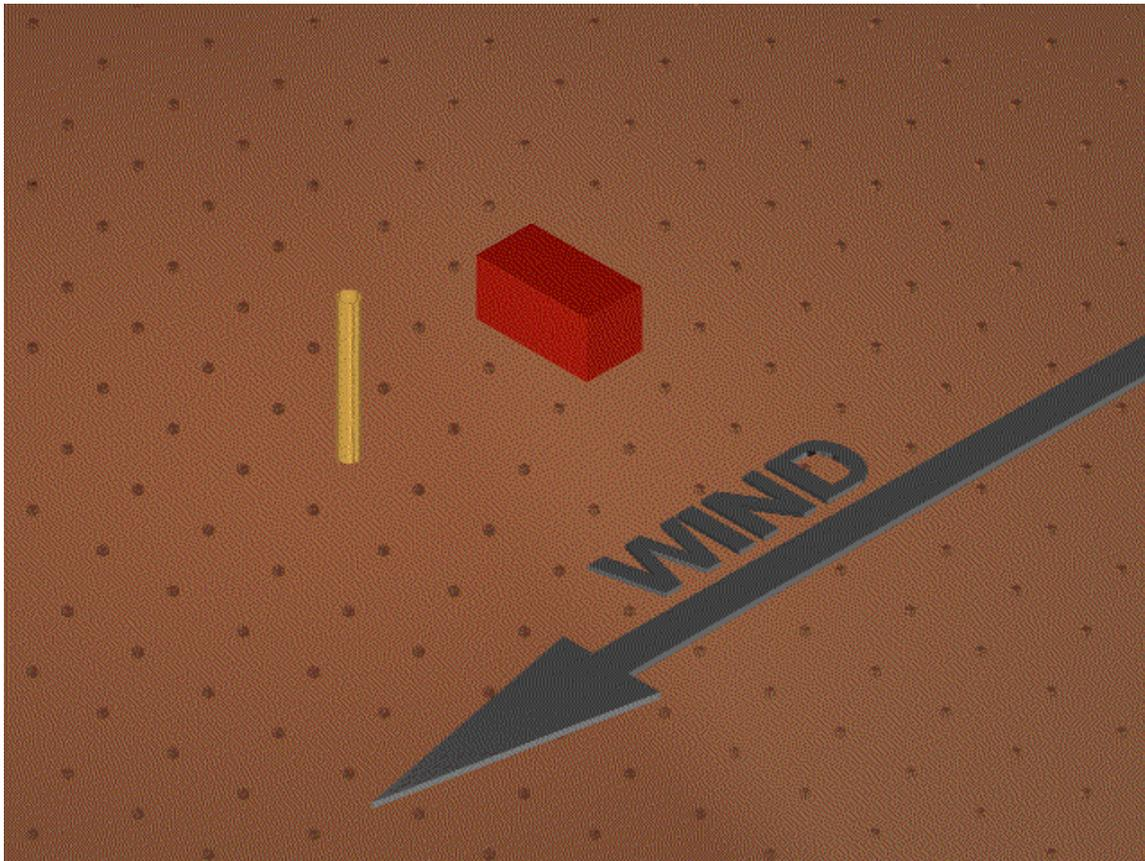
Figure 2. Idealized building and stack configuration for EBD wind tunnel setup.
