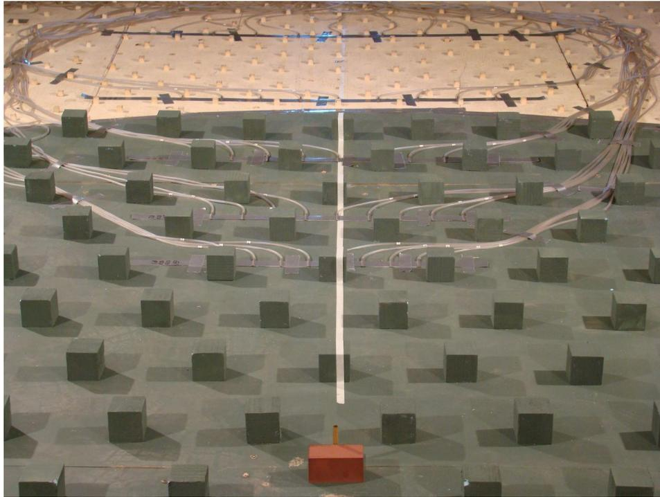
Figure 7. Photograph of a typical ground-level concentration sampling grid.
