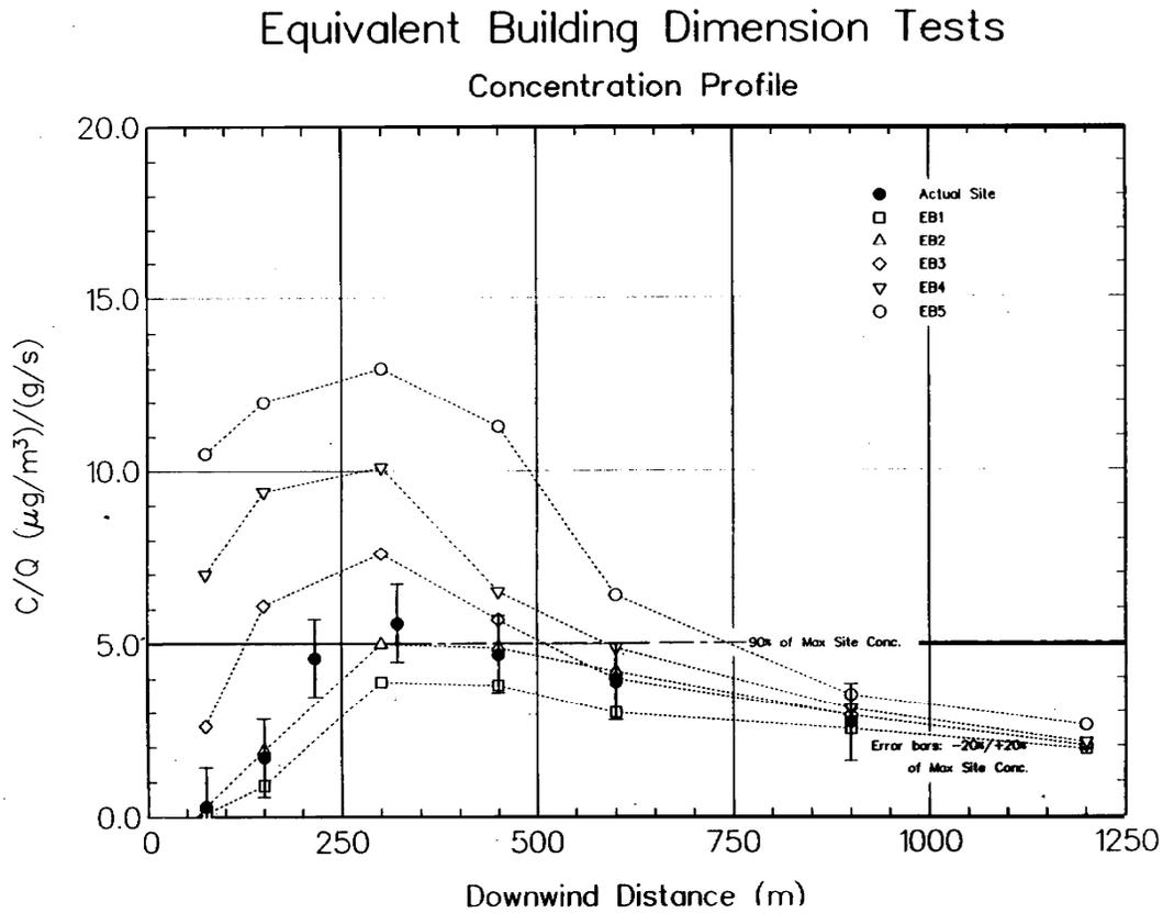
Figure 3. Typical results from a previous equivalent building determination. The figure shows the maximum concentration versus downwind distance with 20 percent error bar with the site structures in place, a horizontal line at 0.9 times the maximum concentration with site structures in place, and maximum concentration versus distance for various equivalent buildings.
