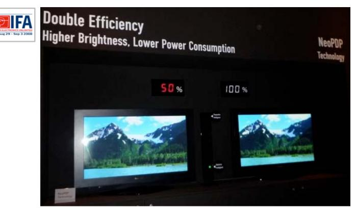
The TV left is the plasma display developed with the "high luminance efficiency technology" and the TV on the right is the 2007 model. Same brightness using half the power.
