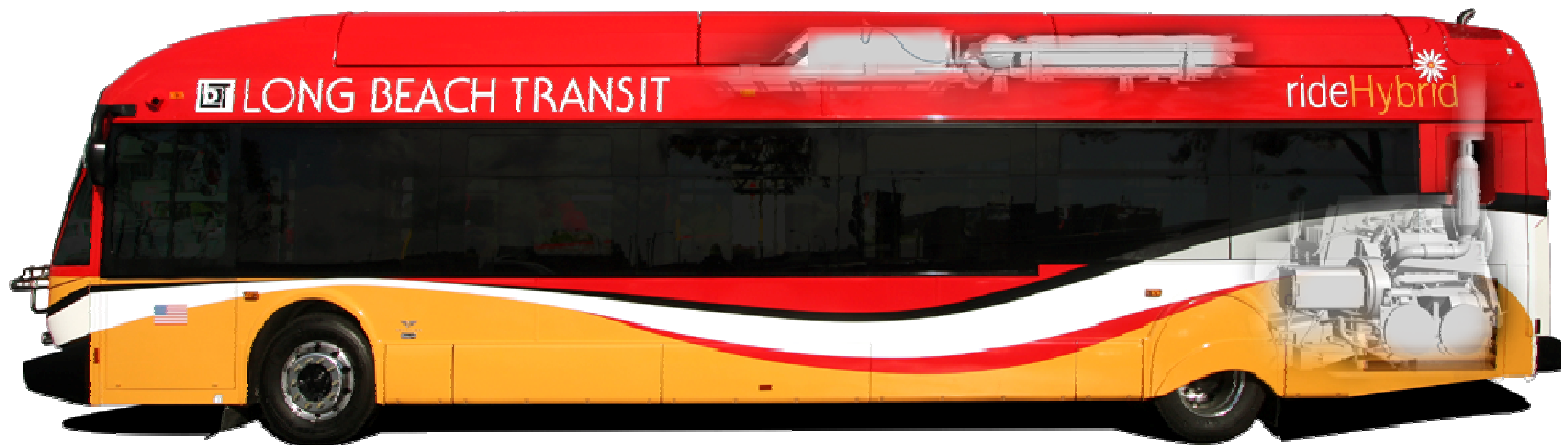
Long Beach Transit operated New Flyer Gasoline Hybrid – “x-ray vision” reveals ultra-capacitors, cooling atop, generator & engine below
