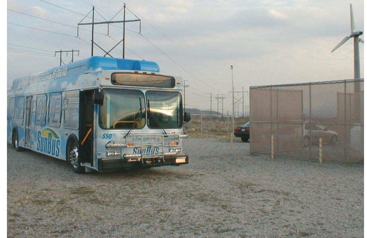
The SunLine Transit HHICE bus, positioned to refuel with hydrogen supplied by wind generation.
