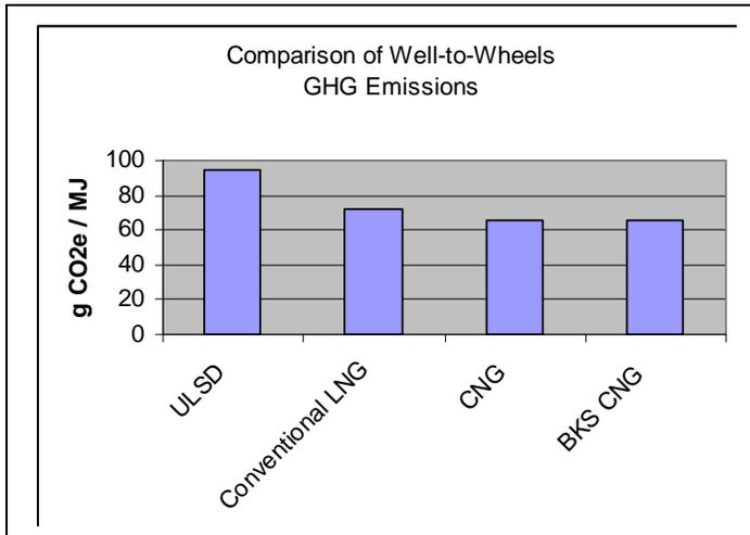
The BKS LNG fuel pathway has a number of promising advantages as a low carbon fuel alternative to ULSD:
