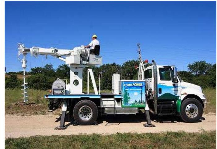
Plug-in Hybrid truck with Digger Derrick
