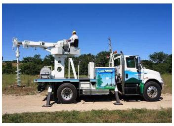
Plug-in Hybrid truck with Digger Derrick
