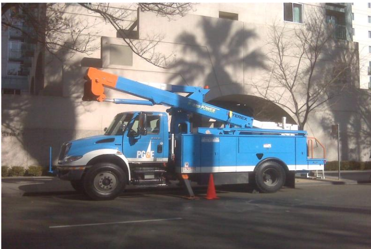
Plug-in hybrid medium-duty truck with Odyne system produced for PG&E
