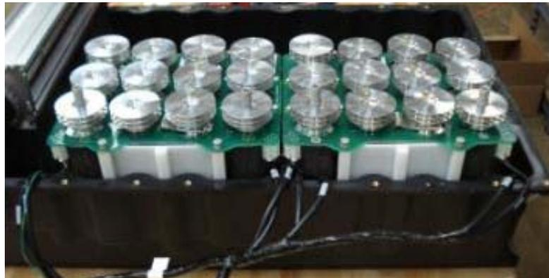
**Figure 1 - This ISE design ultra-capacitor pack is fully sealed and internally cooled with refrigerated liquid.**
