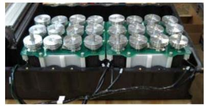
${\bf Figure~1~- This~ISE~design~ultra-capacitor~pack~is~fully~sealed~and~internally~cooled~with~refrigerated~liquid.}$
