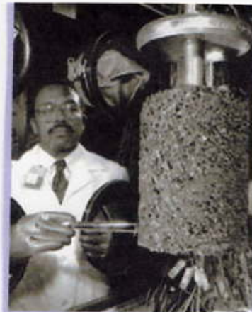
Engineer Eddie Gay inspects uranium that was separated from spent fuel during electrorefining. Argonne National Laboratory photo.
