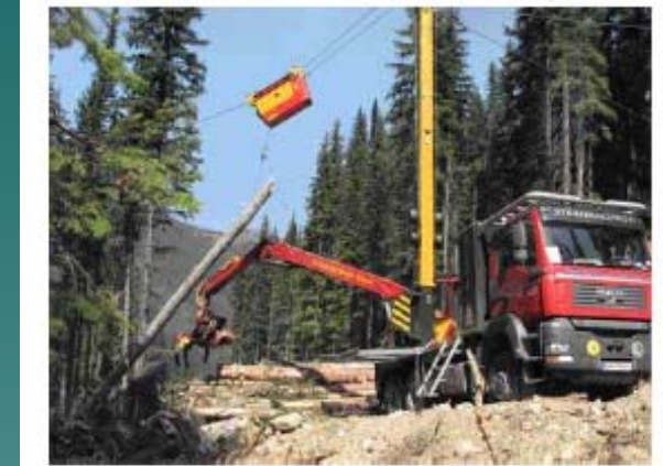
Figure 8. Yarder-processor. Source: McMass Industries
