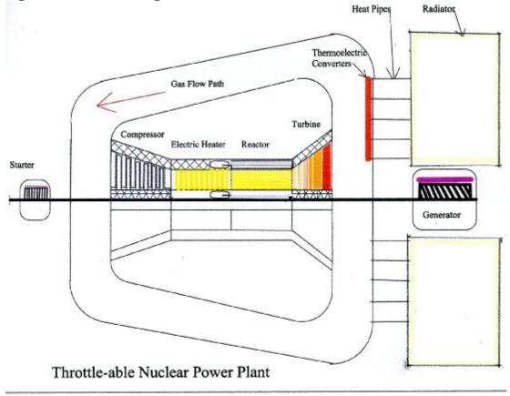
Figure 10. Small 23 Megawatt Gas cooled Throttle-able Nuclear Power Plant
