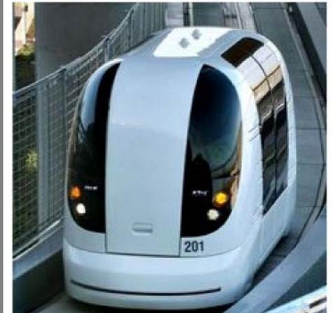
Advanced Transport Systems and BAA Heathrow have commenced running tests on the new ULTra Personal Rapid Transit system that will link the Terminal 5 with a car park on the periphery of the airport.
