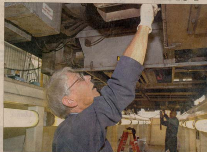
BART MECHANIC Gary Nichols puts a cover back on a line-switch pack Thursday while doing preventive maintenance on a train at the Hayward BART maintenance yard.
