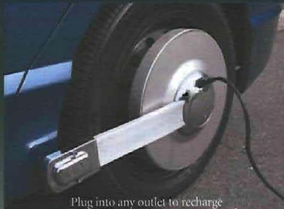
The Poulsen Hybrid installed on a 2006 Honda Civic LX
