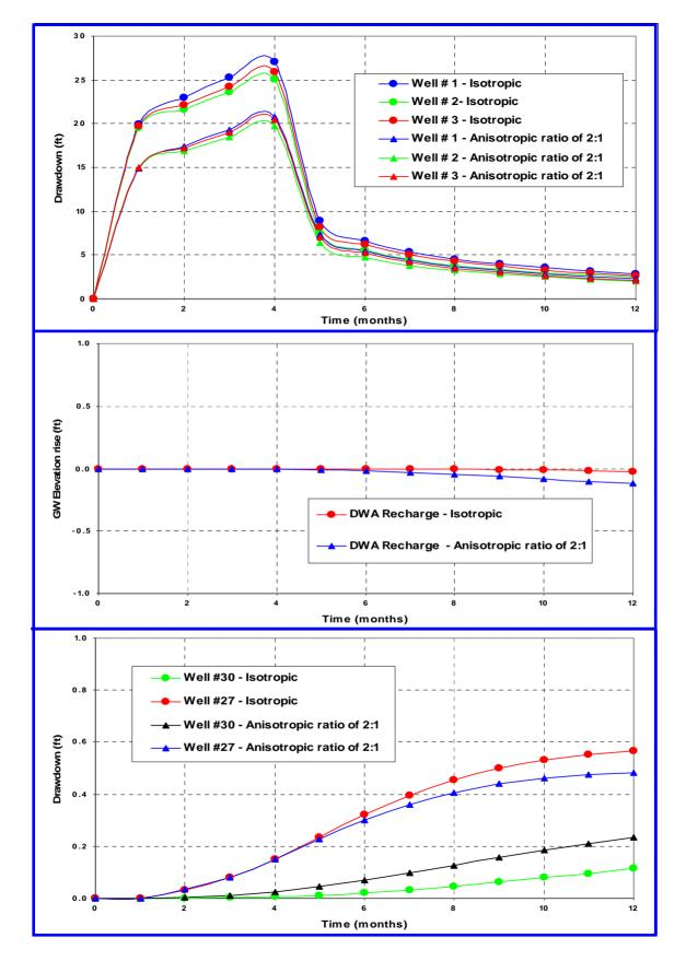
Figure 17: Scenario 3 Results at Project Pumping Wells, DWA Recharge Basin and MSWD Wells 27 and 30 (Pumping = 2,059 gpm, No recharge, Total pumping volume = 1,100 af)
