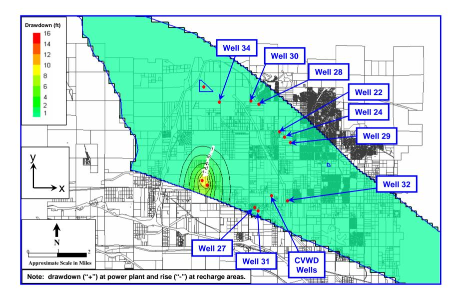
Figure 15: Contour Map of Simulated Groundwater Level Changes at 4 Months – Scenario 3, Anisotropy Ratio =2 (Pumping = 2,059 gpm, No Recharge, Total Volume Pumped = 1,100 af)
