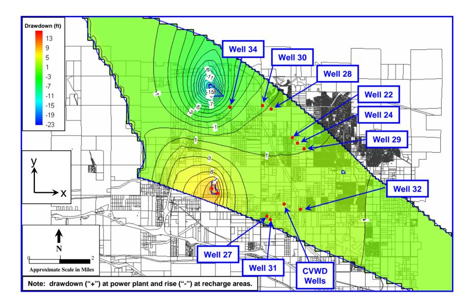
Figure 3: Contour Map of Simulated Groundwater Level Changes at 30 Years – Scenario 1, Anisotropy Ratio =2 (Pumping = 1,100 afy, Recharge = 1,100 afy)
