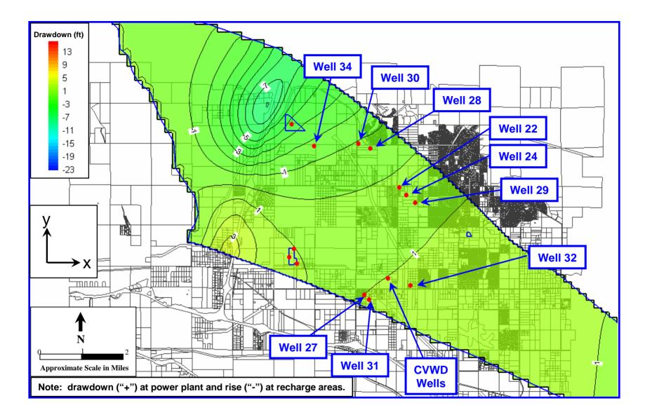
Figure 2: Contour Map of Simulated Groundwater Level Changes at 35 Years – Scenario 1, Anisotropy Ratio =1 (Pumping = 1,100 afy, Recharge = 1,100 afy)
