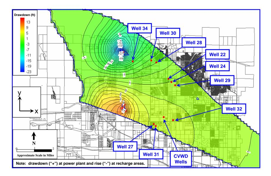
Figure 1: Contour Map of Simulated Groundwater Level Changes at 30 Years – Scenario 1, Anisotropy Ratio =1 (Pumping = 1,100 afy, Recharge = 1,100 afy)
