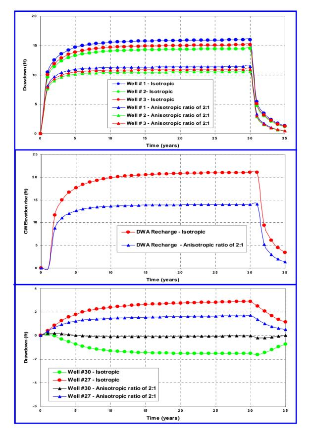
Figure 5: Scenario 1 Results at Project Pumping Wells, DWA Recharge Basin and MSWD Wells 27 and 30 (Pumping = 1,100 afy, Recharge = 1,100 afy)
