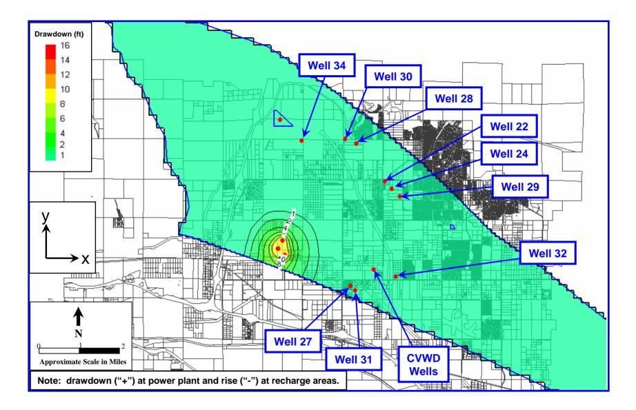
Figure 13: Contour Map of Simulated Groundwater Level Changes at 4 Months – Scenario 3, Anisotropy Ratio =1 (Pumping = 2,059 gpm, No Recharge, Total Volume Pumped = 1,100 af)
