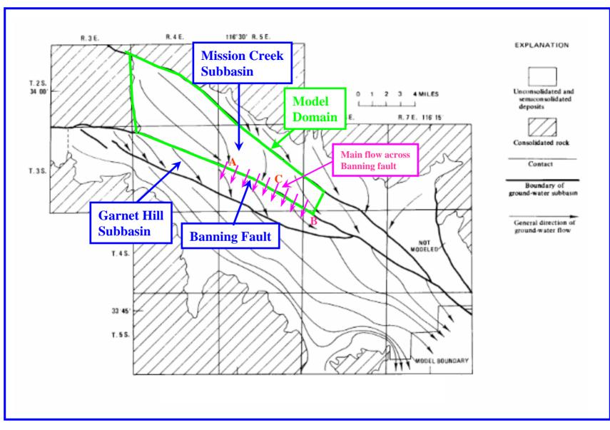
Figure 1: Generalized Groundwater Flow Lines and Section along Banning Fault Where Main Subsurface Outflow Occurs for 1967 (Source: Tyley 1974, Figure 16)
