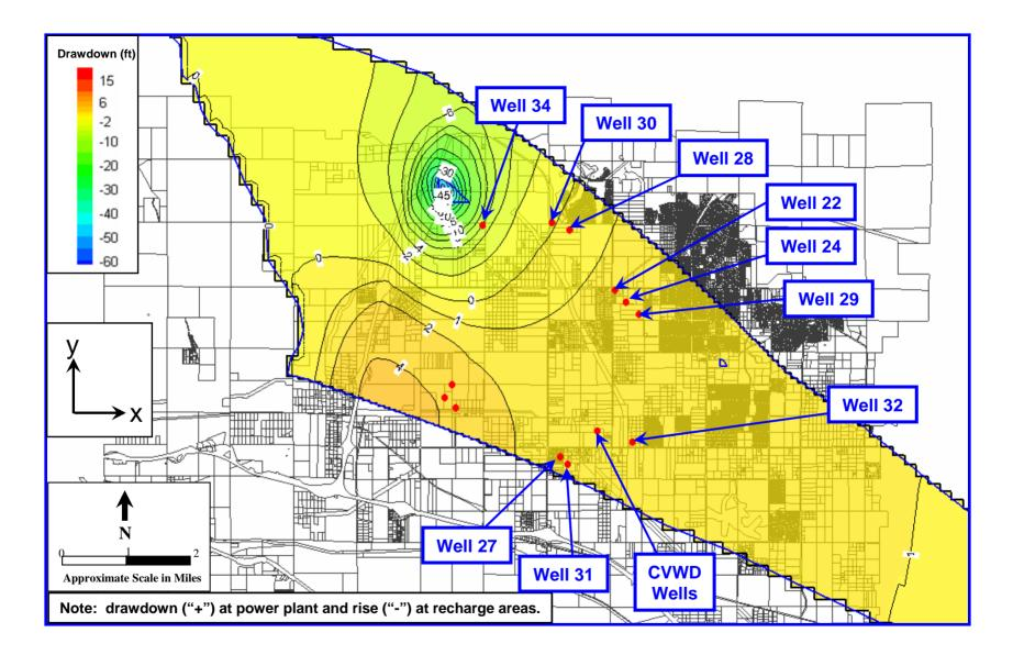
Figure 10: Contour Map of Simulated Groundwater Level Changes at 31 Years – Scenario 2, Anisotropy Ratio =2 Pumping = 1,100 afy, Recharge = 5,500 afy (every 5 years)
