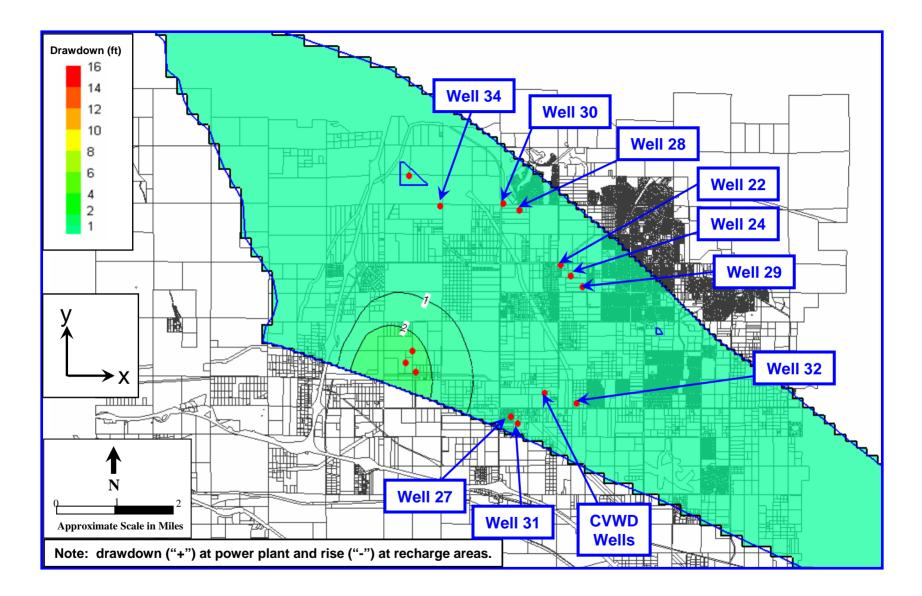
Figure 14: Contour Map of Simulated Groundwater Level Changes at 12 Months – Scenario 3, Anisotropy Ratio =1 (Pumping = 2,059 gpm, No Recharge, Total Volume Pumped = 1,100 af)
