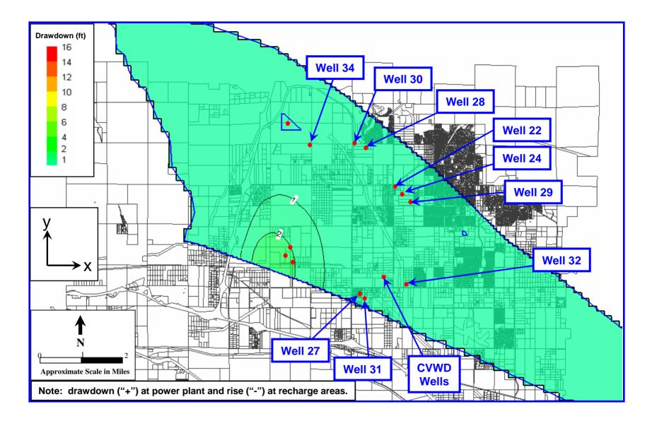
Figure 16: Contour Map of Simulated Groundwater Level Changes at 12 Months – Scenario 3, Anisotropy Ratio =2 (Pumping = 2,059 gpm, No Recharge, Total Volume Pumped = 1,100 af)
