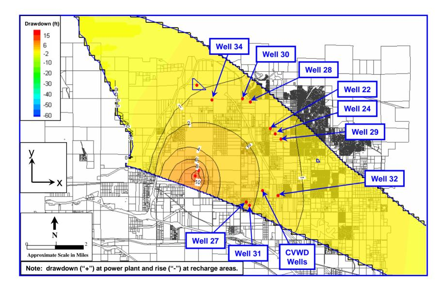
Figure 6: Contour Map of Simulated Groundwater Level Changes at 5 Years – Scenario 2, Anisotropy Ratio =1 Pumping = 1,100 afy, Recharge = 5,500 afy (every 5 years)
