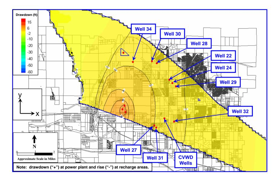
Figure 9: Contour Map of Simulated Groundwater Level Changes at 5 Years – Scenario 2, Anisotropy Ratio =2 Pumping = 1,100 afy, Recharge = 5,500 afy (every 5 years)
