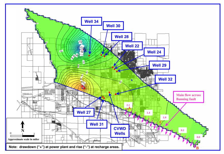
Figure 5: Contour Map of Simulated Groundwater Level Changes at 30 Years – Scenario 1, Anisotropy Ratio =1 (Tyley T, Pumping = 1,100 afy, Recharge = 1,100 afy)
