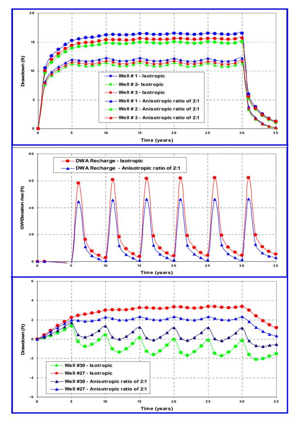
Figure 12: Scenario 2 Results at Project Pumping Wells, DWA Recharge Basin and MSWD Wells 27 and 30 (Pumping = 1,100 afy, Recharge = 5,500 afy every 5 years)
