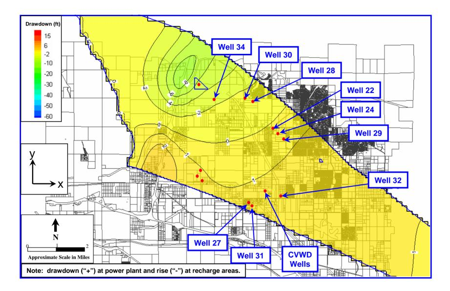
Figure 8: Contour Map of Simulated Groundwater Level Changes at 35 Years – Scenario 2, Anisotropy Ratio =1 Pumping = 1,100 afy, Recharge = 5,500 afy (every 5 years)
