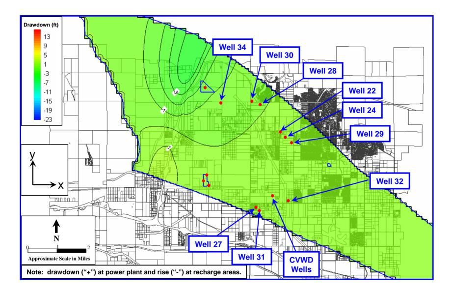
Figure 4: Contour Map of Simulated Groundwater Level Changes at 35 Years – Scenario 1, Anisotropy Ratio =2 (Pumping = 1,100 afy, Recharge = 1,100 afy)
