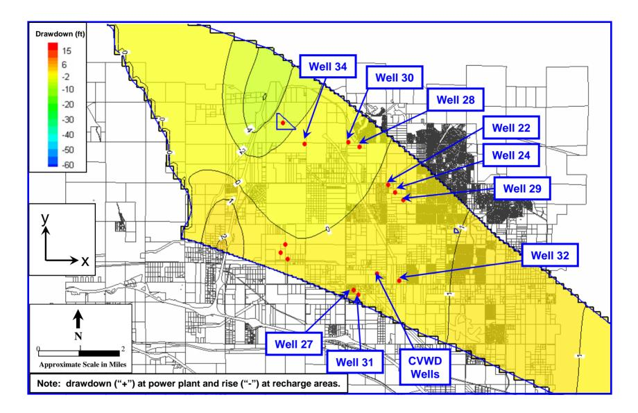
Figure 11: Contour Map of Simulated Groundwater Level Changes at 35 Years – Scenario 2, Anisotropy Ratio =2 Pumping = 1,100 afy, Recharge = 5,500 afy (every 5 years)
