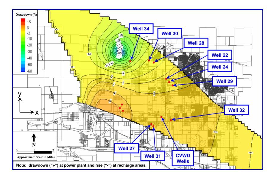
Figure 7: Contour Map of Simulated Groundwater Level Changes at 31 Years – Scenario 2, Anisotropy Ratio =1 Pumping = 1,100 afy, Recharge = 5,500 afy (every 5 years)
