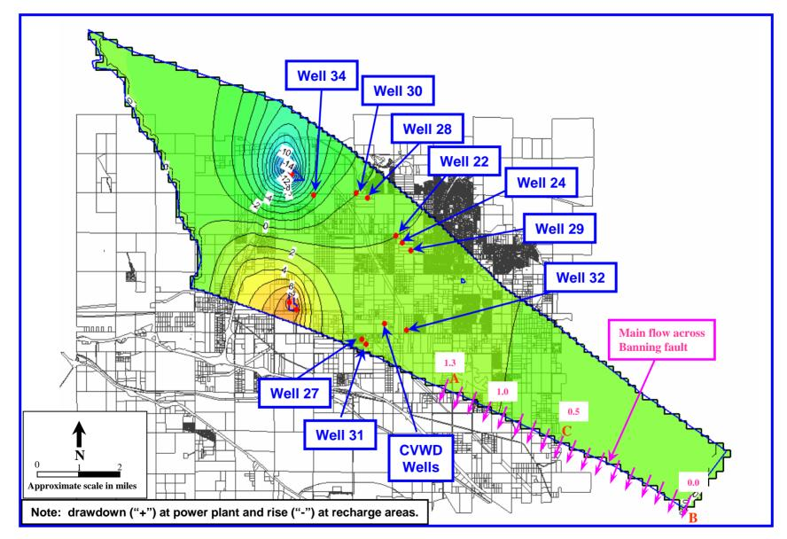
Figure 4: Contour Map of Simulated Groundwater Level Changes at 30 Years – Scenario 1, Anisotropy Ratio =2 (Tyley T, Pumping = 1,100 afy, Recharge = 1,100 afy)
