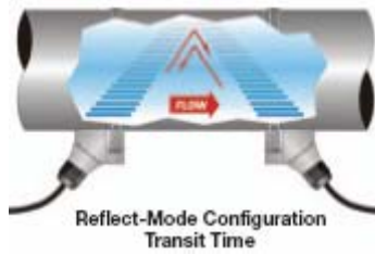
Diagram depicting the sound energy transmission between the transducers (Dynasonics 2006)
