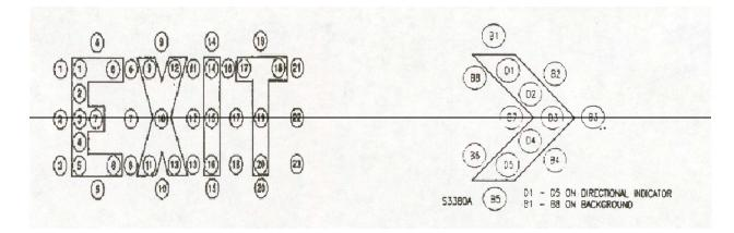
The luminance for each numbered position in the legend and directional indicator shall be measured over a circular area as large as possible while maintaining at least a 1.6 mm distance between the perimeter of the circular area and the adjacent border. The positions for measuring the luminances of the background shall lie within 25.4 mm of the legend and directional indicator but no closer than 1.6 mm to the border.
