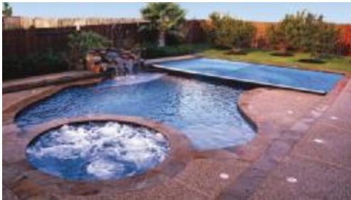
Figure 5. Picture of an automatic pool cover with permanently mounted tracks underneath the deck. Source: www.coverpools.com
