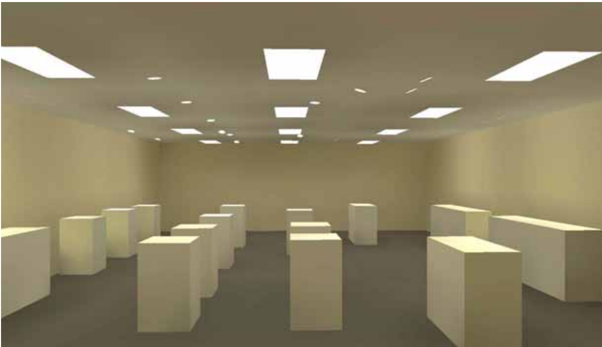
Figure 6: Model E1 Small strip mall retail business (Card Shops, Flower Shop, Hobby Store) using 2x4 T8 recessed luminaires for ambient lighting
