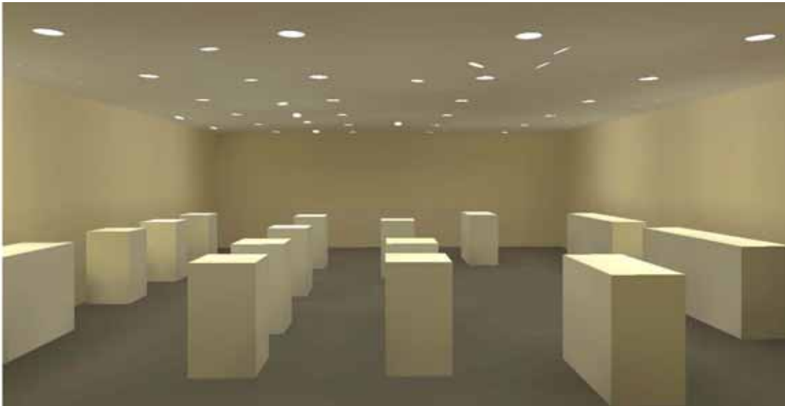
Figure 5: Model E Small strip mall retail business (card Shops, flower Shop, hobby store) using 42W recessed CFL luminaires for ambient lighting
