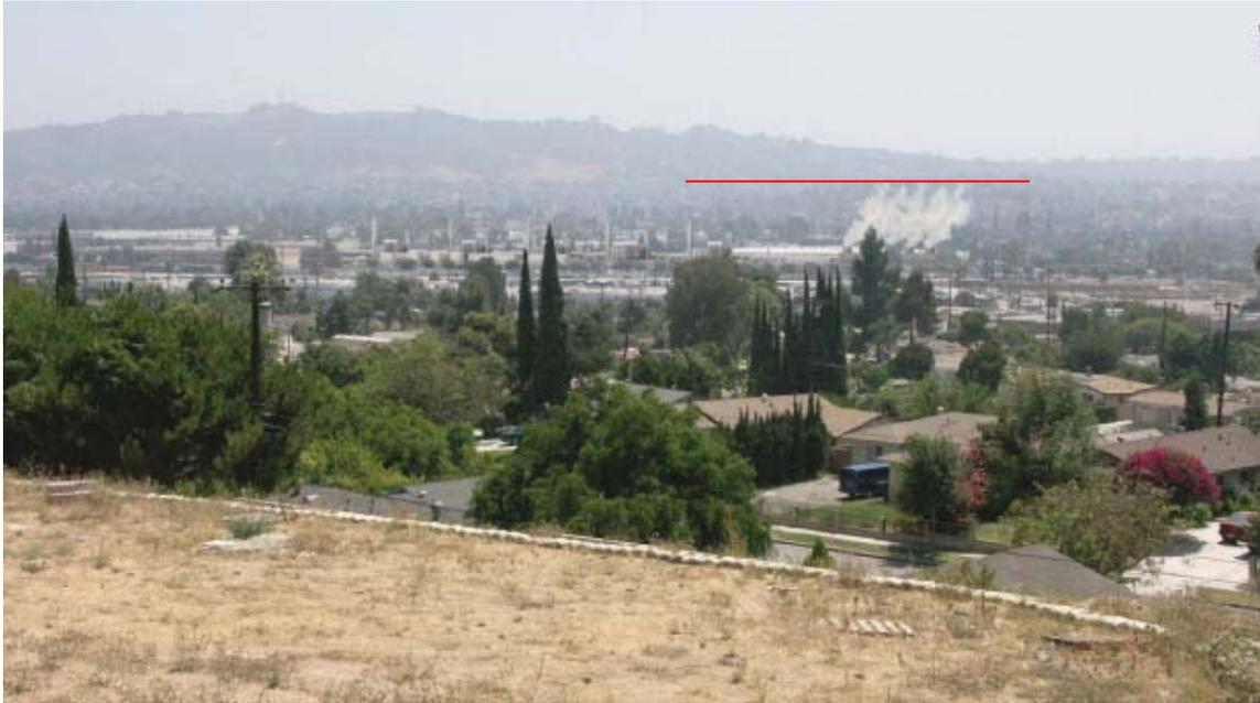
As shown in the photo-simulation, the winter plume dimensions would be slightly larger than summer plumes. The predicted plume size is taken from the base of the cooling tower stack, and is predicted to be 125 feet tall and 74 feet long. (FSA, 4.12-10.)
