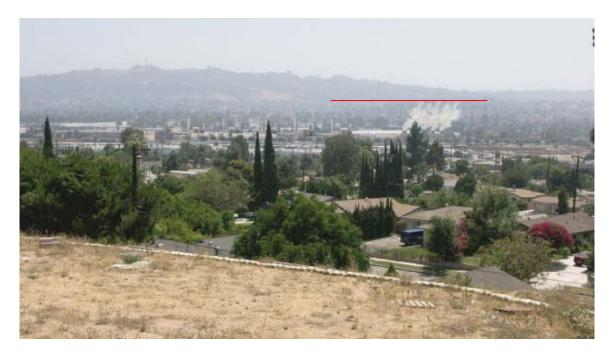
As shown in the photo-simulation, the winter plume dimensions would be slightly larger than summer plumes. The predicted plume size is taken from the base of the cooling tower stack, and is predicted to be 125 feet tall and 74 feet long. (FSA, 4.12-10.)
