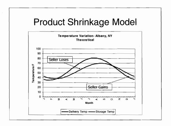
Explain source of the curve data: blue from temperature on terminal rack meter tickets and purple form temperature sensor on underground monitoring system.
