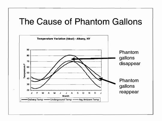
Phantom gallons is a universal problem for the retailer with underground tanks. Inventory losses at some time of the year and gains in other parts of the year. They are somewhat predictable based on the temperature differential between the supply tank and the underground tank. More gallons disappear than appear since the differentials are different.
