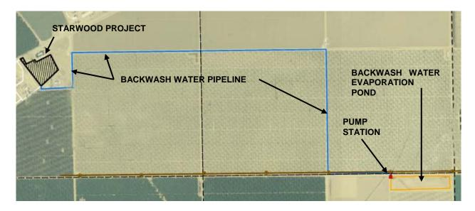
When the water pumped to the SPP from the backwash pond reaches the site it will be sent through a sand filter to remove any solid debris or other particulate materials in the water. The water will then be routed from the sand filter to the reverse osmosis (RO) unit. In addition to storm water runoff, an on-site unlined evaporation pond will collect discharge wastewater from the RO unit as well as periodic sand filter backwash. (Alt. Water Supply Analysis, 1-3)
