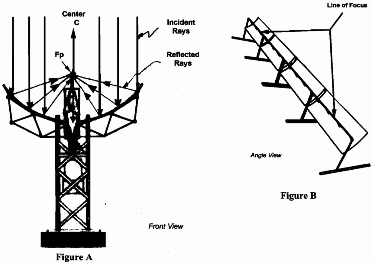
A parabolic reflective surface (Figure A) will precisely direct an Incident Ray of light (Ir) to a focal point (Fp)  $\frac{1}{2}$  the distance from the center (C) of the arc. There is a "line of focus" (Figure B) created by the parabolic trough that will travel the full length of the mirror.
