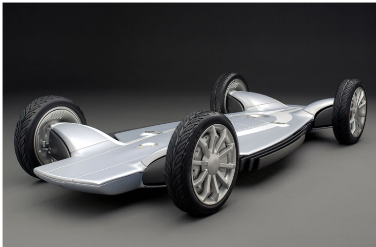
Figure 5-3: GM AUTOnomy Concept Skateboard Chassis 37
