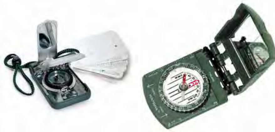
Figure 4 – Compass with a sighting feature
