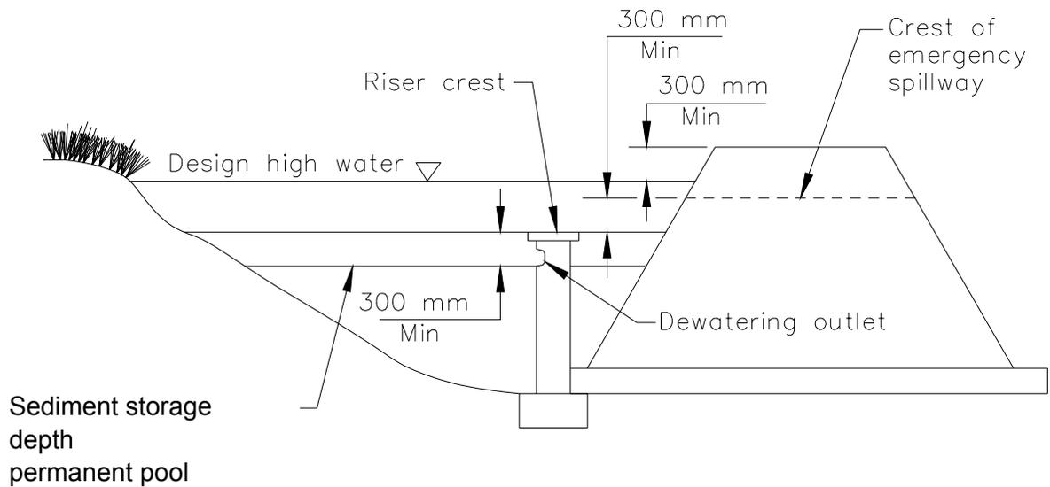
This outlet provides no drainage for permanent pool.
