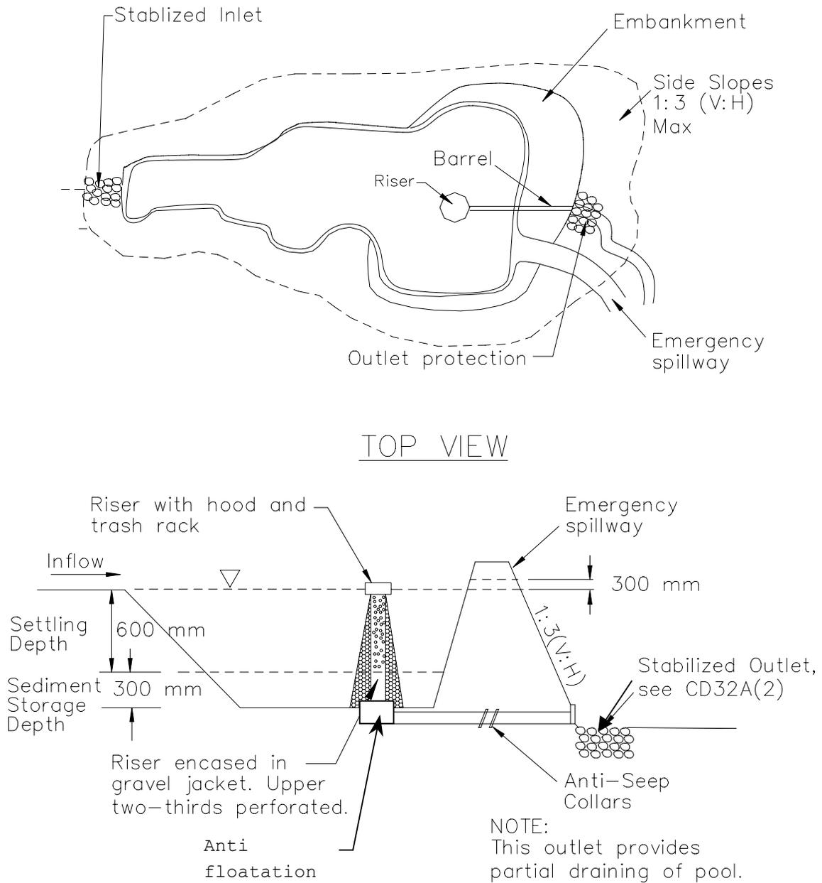
**FIGURE 2: MULTIPLE ORIFICE DESIGN**
