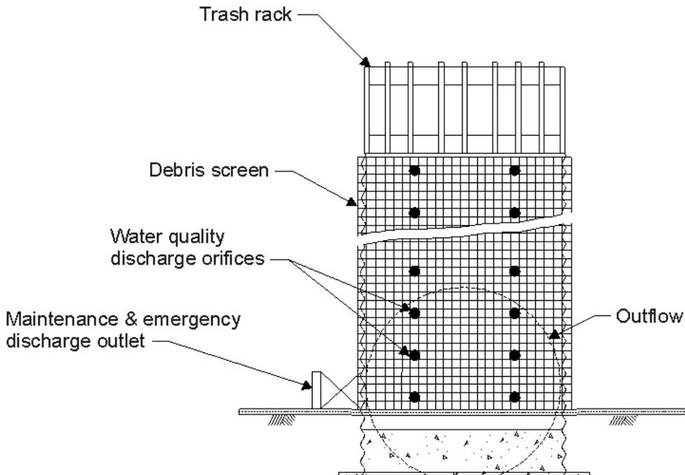
**FIGURE 3: MULTIPLE ORIFICE OUTLET RISER
