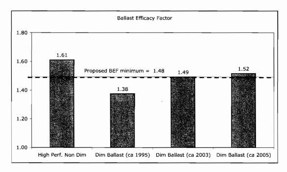
This level would just allow the (2003) dimming ballast and definitely the new Sylvania product (BEF = 1.52). However, it would exclude the dimming ballast (1995) as too inefficient.
