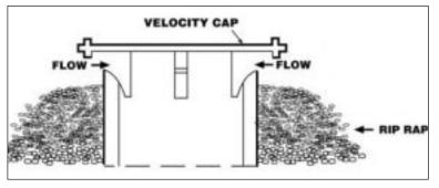
discharge structures for El Segundo Units 3 and 4.
