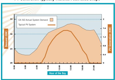
Figure 13 PV Generation Typically Matches Peak Load Shape
