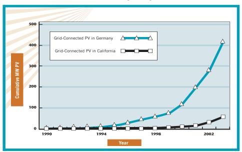
Figure 12 Grid-Connected PV: Germany Compared to California
