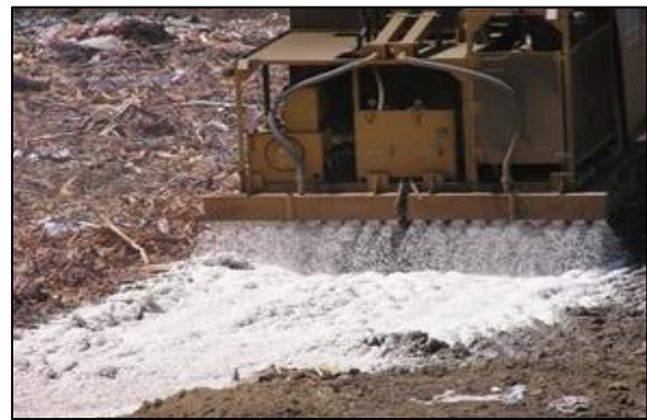
Figure 24 - Spray-on Foam ADC.
