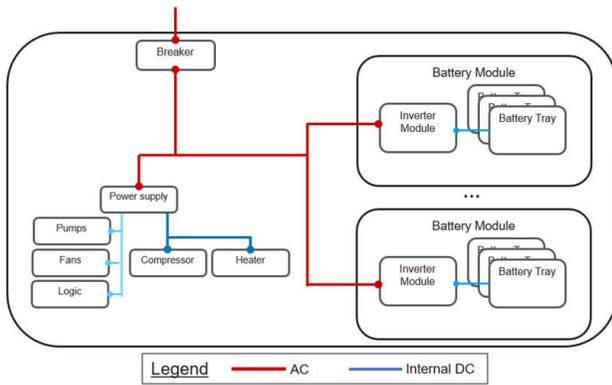
Figure 2-3 - Battery Module
