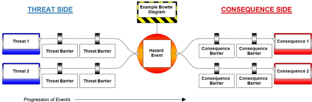
Each fault condition per *NFPA 855* and *IFC* assessed in Sections 3.4.1 – 3.4.6 below is accompanied by a corresponding bowtie diagram indicating critical *threat* and *consequence* pathways and the mitigative barriers between them. As the most critical risk posed by lithium-ion battery cells comes from the propagation of thermal runaway from a failing cell (or multiple cells) to surrounding cells, this serves as the primary critical hazard for the subsequent failure scenarios.
