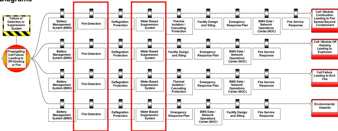
**Table 3-7 - Failure of Smoke Detection, Fire Detection, Fire Suppression, or Gas Detection System Barriers**
