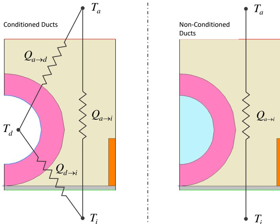
**Figure 12: Left-hand picture depicts a heat transfer network representing a buried duct inside attic blown-in insulation and resting on top of the ceiling drywall. Right-hand picture represents the same case but with no conditioned air running through the ducts.**
