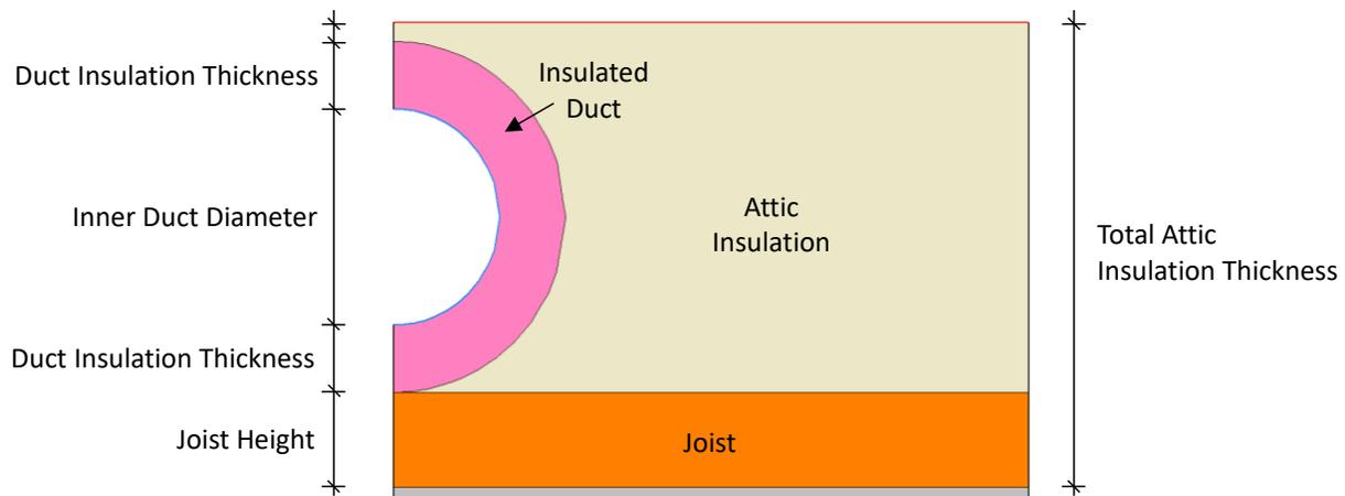
**Figure 2: Insulated ducts buried within loose-fill attic insulation.**
