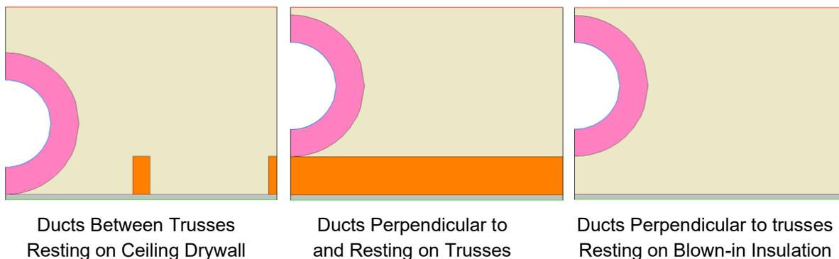
**Figure 4: Simulation cases to represent location of ducts buried in insulation.**
