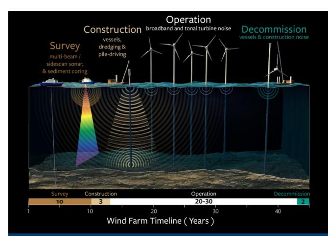
**Figure 2.** Underwater noise associated with the life cycle of an OSW farm area, including during site surveys, construction, operations and maintenance, and decommissioning. Illustration from <u>Mooney et al. (2020).</u>
