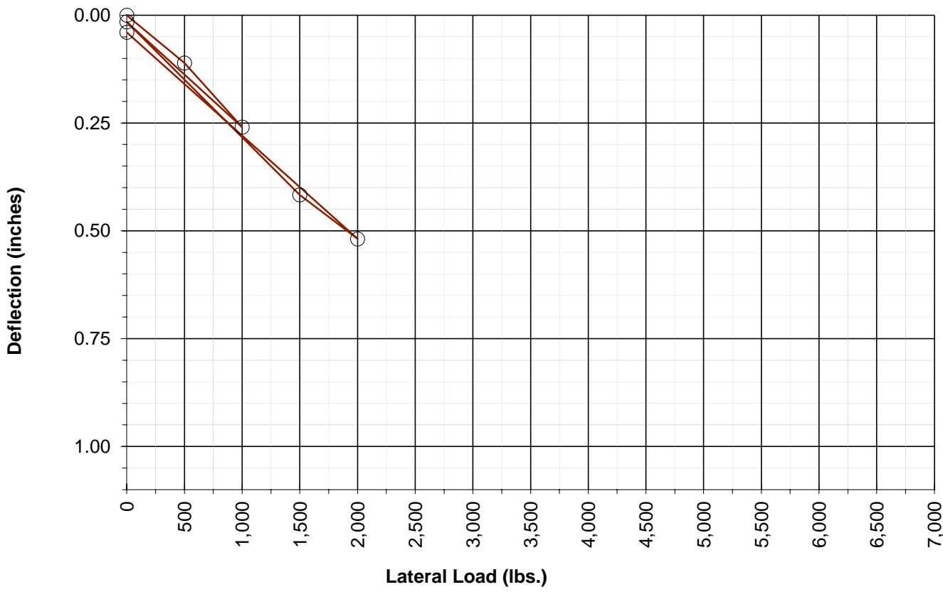
—○— Lateral - Gauges at 6-inches above ground surface
