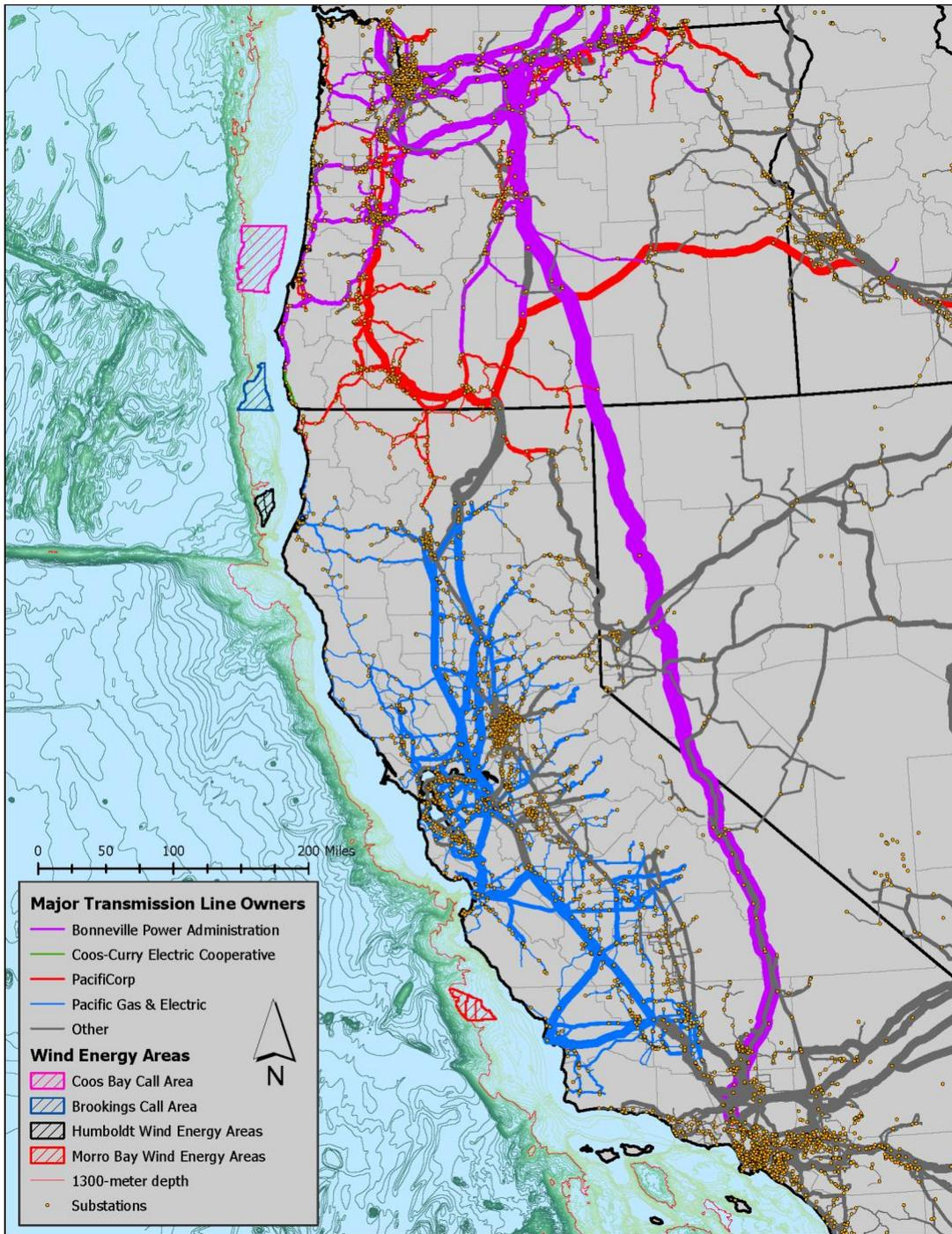
**Figure 2. Existing transmission infrastructure and officially delineated BOEM “Call” or “Wind Energy Areas” in California and southern Oregon.<sup>2</sup> Line thickness corresponds to line voltage.**
