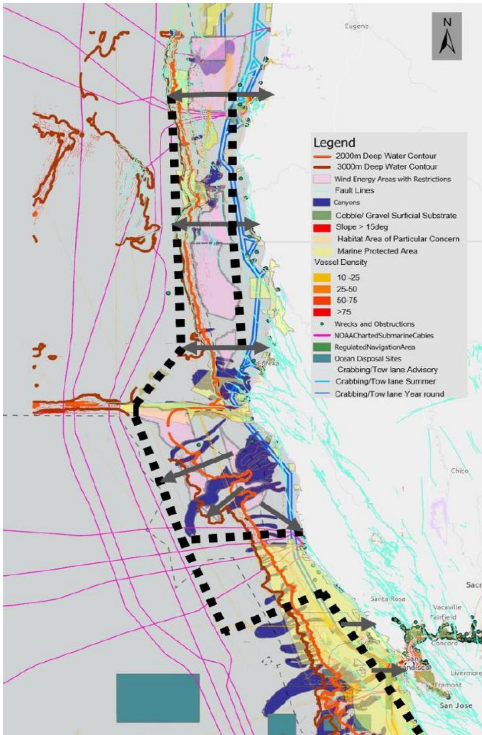
**Figure 7. Summary of subsea constraints and example conceptual large-scale transmission corridors<sup>7</sup>.**
