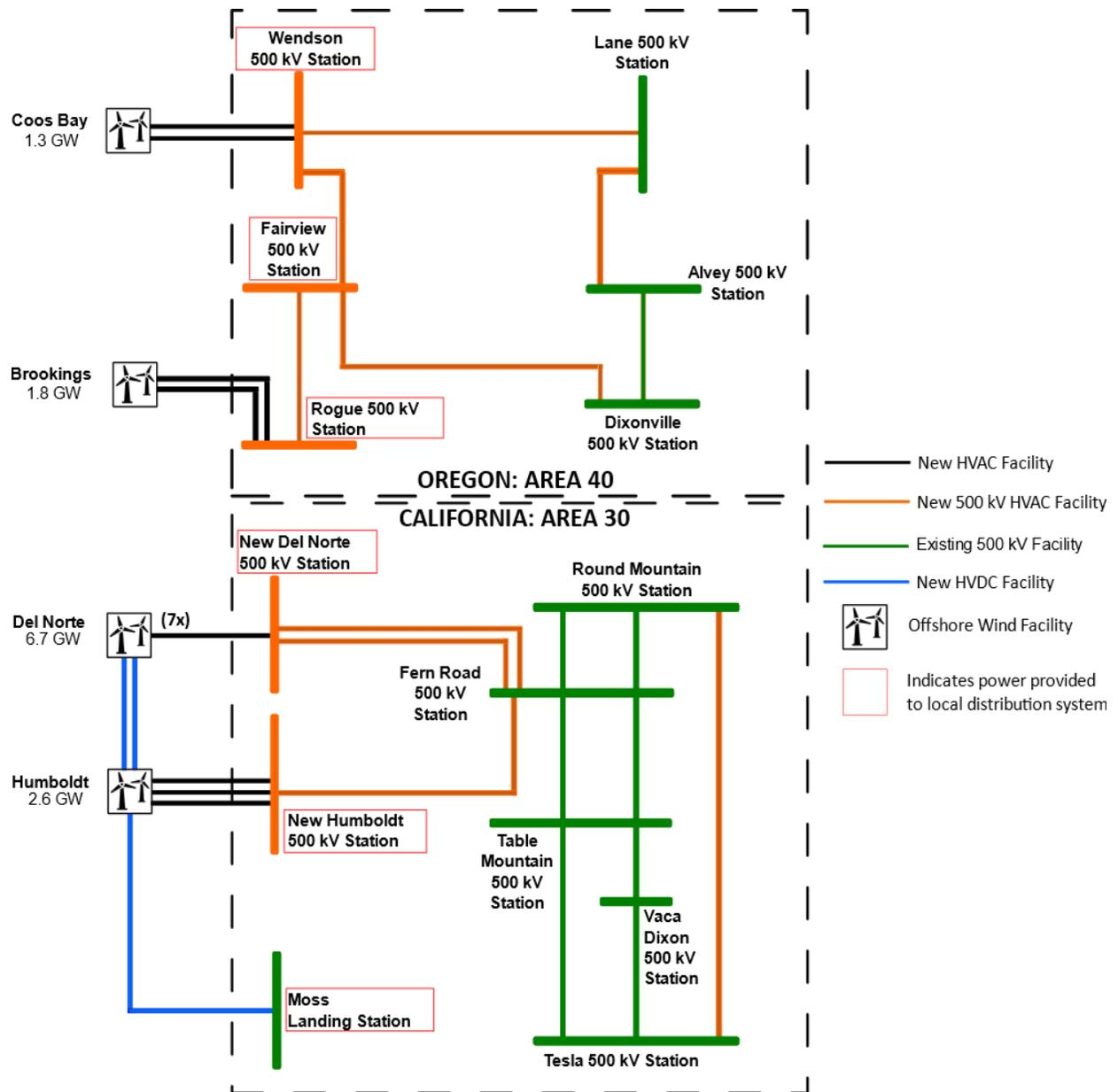
Figure 10. Single line electrical schematic for Alternative 12.4c
