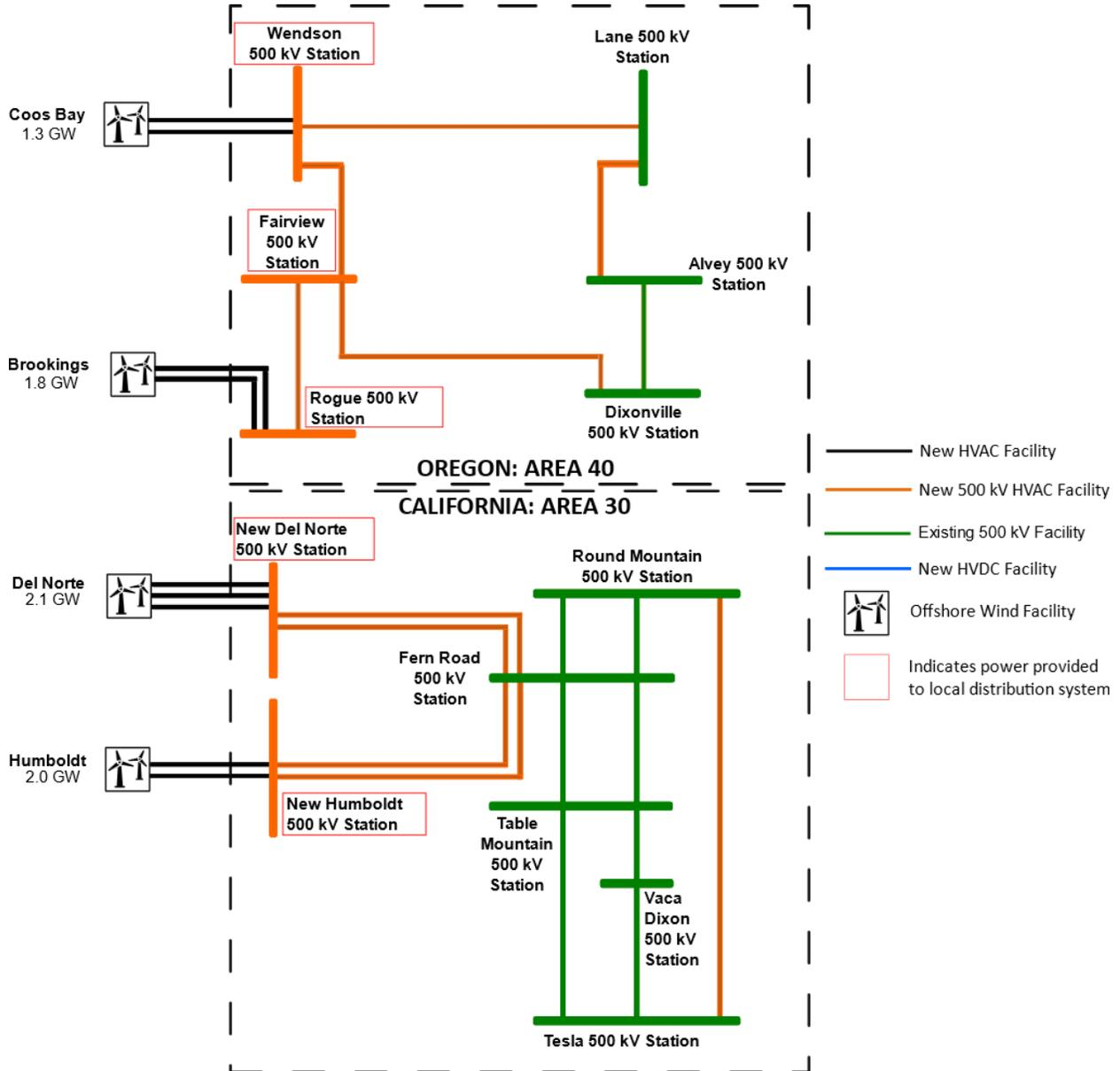
Figure 8. Single line electrical schematic for Alternative 7.2a
