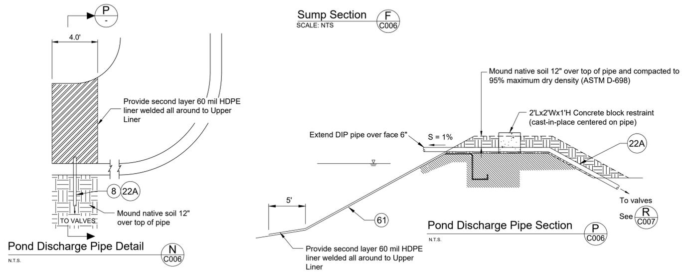
**Pond Discharge Pipe Detail** (N C006)
