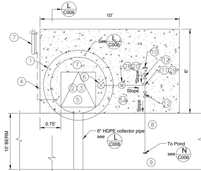
LCRS Collection Manhole and Concrete Pad Detail
