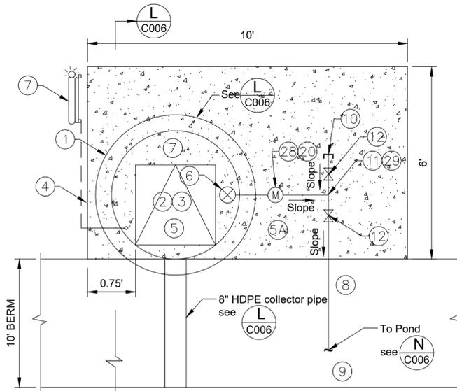
**LCRS Collection Manhole and Concrete Pad Detail** (M C007)
