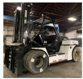
Source: Wiggins, battery electric forklift
