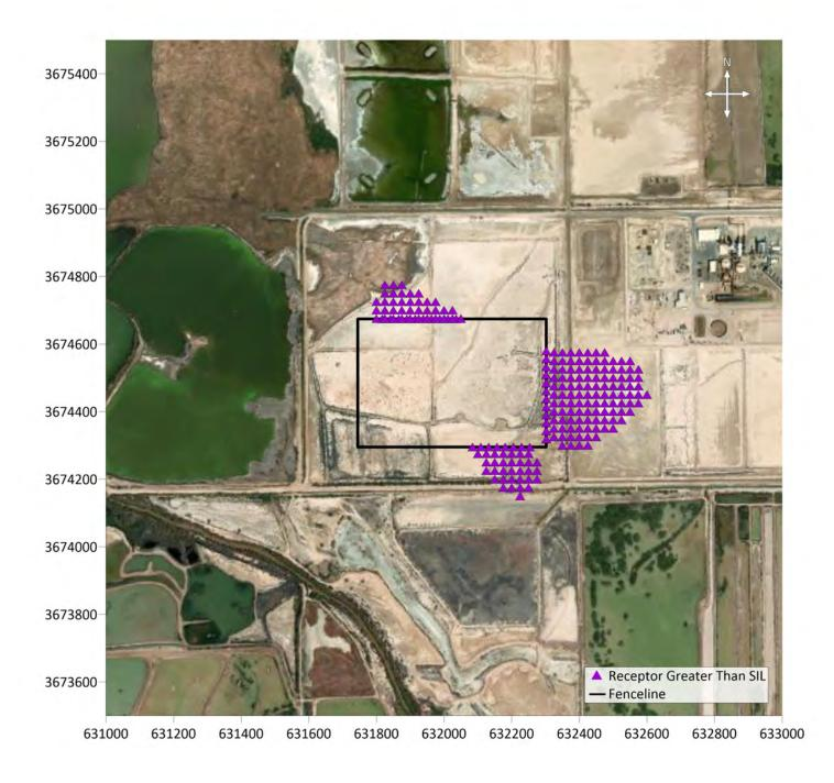
Figure A-6: Morton Bay Operation Annual PM<sub>2.5</sub> Significant Impact Radius
