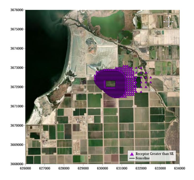
Figure B-6: Elmore North Construction Annual PM<sub>2.5</sub> Significant Impact Radius
