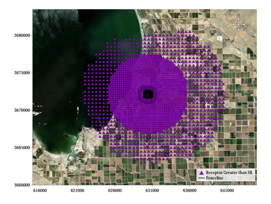
Figure B-5: Elmore North Construction Annual NO<sub>2</sub> Significant Impact Radius
