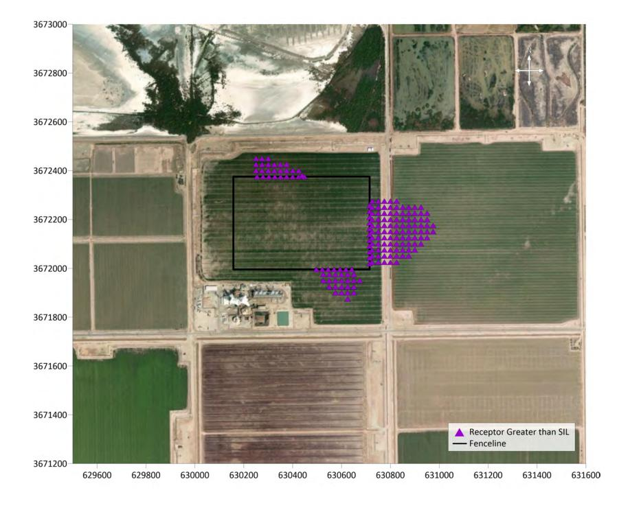
Figure A-4: Elmore North Operation Annual PM<sub>2.5</sub> Significant Impact Radius
