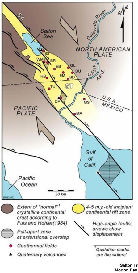
Figure DRR 9a-1 Salton Trough Tectonic Map, Morton Bay Geothermal Project Imperial County, California
