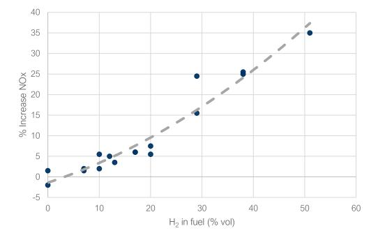
GE extrapolates that gas turbine NOx emissions could potentially double if operating at or near 100% hydrogen.
