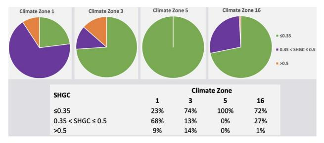
Figure 2: Percentage of windows installed in Climate Zones 1, 3, 5, and 16 with a solar heat gain coefficient of less or equal to 0.35, larger than 0.35 but less or equal to 0.5, or larger than 0.5.
