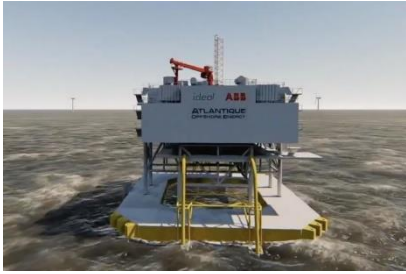
Ideol and AOE's (barge) design based on Ideol's shallow-draft Damping Pool concept 36
